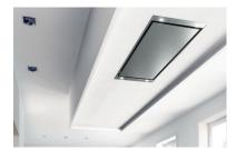
Cooking vapours do not rise straight up, instead they fan out over an angle of between 10° and 15°. For an efficient operation it is important that the whole construction in which the ceiling unit is installed is at least the same width and depth as the hob. Create an overlap of approximately 30 cm around the ceiling unit to prevent cooking vapours from escaping. In addition, edging of 5 to 10 cm high will ensure that fewer vapours can escape.
