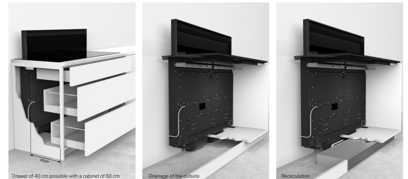
Drawer of 40 cm possible with a cabinet of 60 cm
